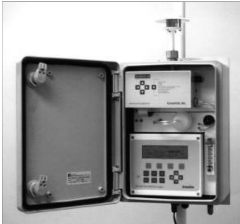
The Model ES-640 Digital Particulate Monitor is for continuous monitoring and recording.
